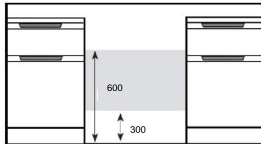
Gas hose connection point must be installed within the shaded area
