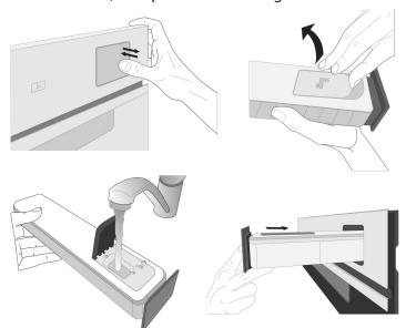
After the first filling, in case of longer cooking cycles, once water will have ran out, it could be necessary to add it again, in order to complete the cycle: the oven will prompt it in case it is needed.
