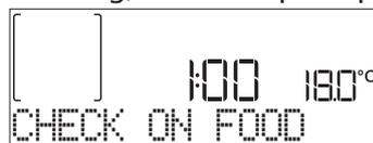
An audible signal will sound and the display shows the action to be done. Check the food, close the door and press or to continue cooking.
