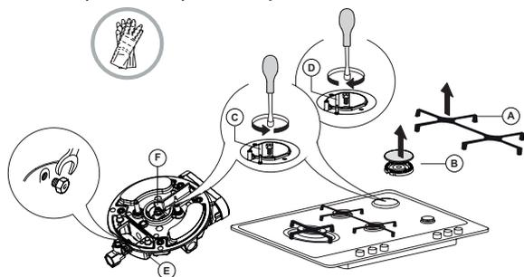
Before installing the hob, remember to affix the gas calibration plate supplied with the injectors in such a way that it covers the existing information relating to gas calibration.
