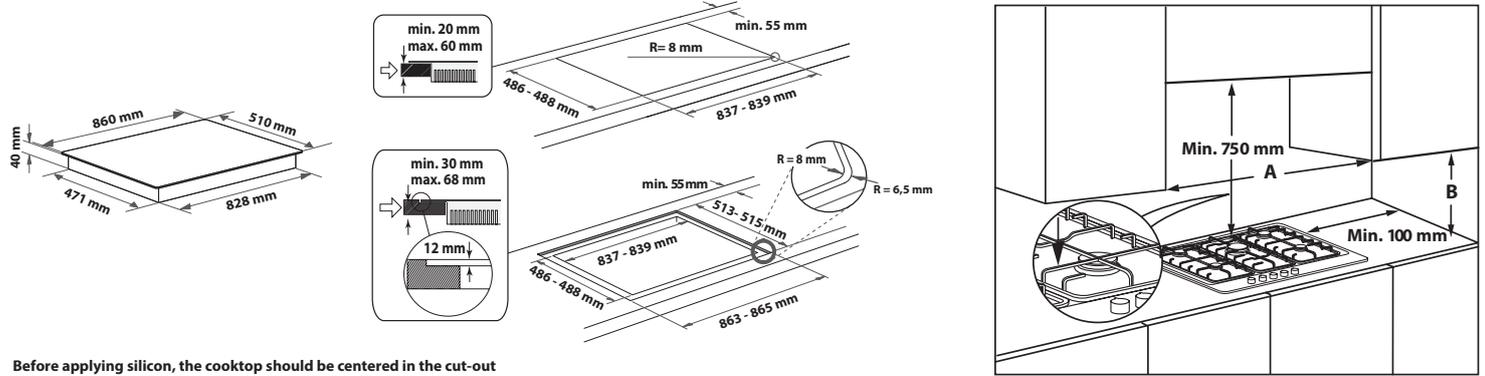
Before applying silicon, the cooktop should be centered in the cut-out
