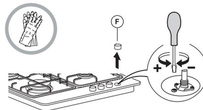
Upon completion of adjustment, reseal using sealing wax or an equivalent material.
