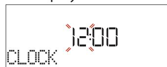
Press + or — to set the current hour and press ✓ : The two digits for the minutes will flash on the display.
