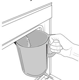
Once selected the "Drain" function, press ▶ and follow the actions indicated: Open the door and place a large jug under the drain nozzle located at the bottom right of the panel. Once started the draining, keep the jug in position until the operation is completed.
