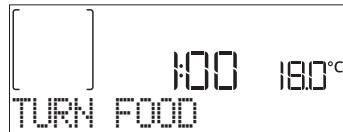
An audible signal will sound and the display shows the action to be done. Open the door, do the action prompted by the display and close the door, then press **►** to continue cooking.
