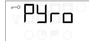
Once the cycle has been completed, the door remain locked until the temperature inside the oven has returned to a safe level. Air the room during and after running the Pyro cycle.
