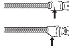
For water stop hoses: check the small safety valve inspection window (see arrow). If it is red, the water stop function was triggered, and the hose must be replaced by a new one. For unscrewing this hose, press the release button (if available) while unscrewing the hose.
