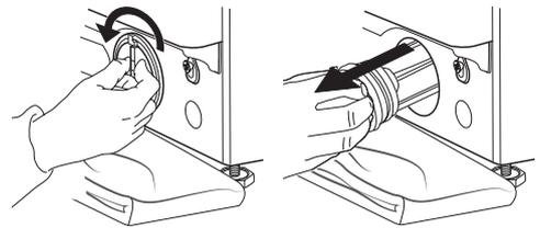
5. Clean the water filter: remove residues in the filter and clean it under running water.
