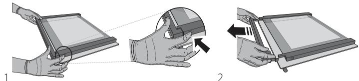
Lift and firmly hold the inner glass with both hands, remove it and place it on a soft surface before cleaning it (3).
