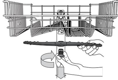
To remove the upper spray arm, turn the plastic locking ring in a clockwise direction. The upper spray arm should be replaced so that the side with the greater number of holes is facing upwards.
