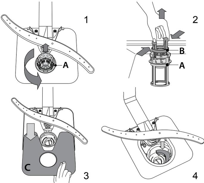
After cleaning the filters, re-place the filter assembly and fix it in position correctly; this is essential for maintaining the efficient operation of the dishwasher.
