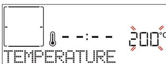
When the value flashes on the display, press + or — to change it, then press ✓ to confirm and continue with the settings that follow (if possible).
