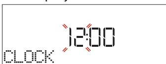
Press + or — to set the current hour and press ✓ : The two digits for the minutes will flash on the display.
