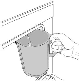
Once selected the "Drain" function, press **►** and follow the actions indicated: Open the door and place a large jug under the drain nozzle located at the bottom right of the panel. Once started the draining, keep the jug in position until the operation is completed. The average duration for full load drainage is about three minutes.
