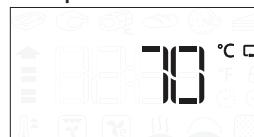
If the meat probe is plugged during the selection of a function, display switches to the default meat probe target temperature.
