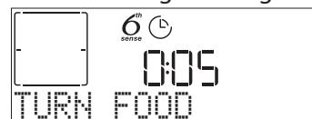
An audible signal will sound and the display shows the action to be done. Open the door, do the action prompted by the display and close the door.
