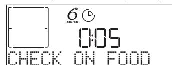
An audible signal will sound and the display shows the action to be done. Check the food, close the door and press
