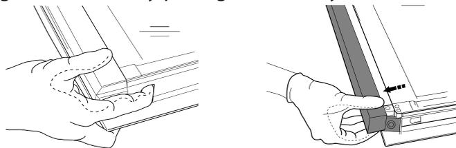
**2.** Lift and firmly hold the inner glass with both hands, remove it and place it on a soft surface before cleaning it.
