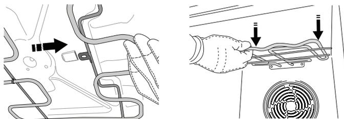
**2.** To return the heating element to its position, lift it up, pull it slightly towards you and make sure that the tab support is in its proper seating.
