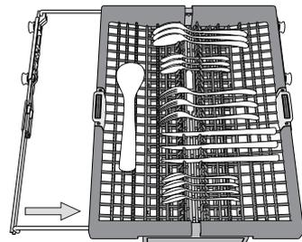
The cutlery basket is equipped with two sliding side trays to make the most of the height of the space below and enable the loading of high items into upper rack.
