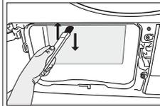
You can use a vacuum cleaner with a brush for cleaning. If the vacuum cleaner does not have a brush, it is not recommended to be used for condenser cleaning.
