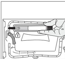
Pull the brush to the left to remove it. You can use the cleaning brush to clean filter, condensing metal surface and accumulated fibre on the door.
