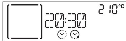
Notes: Programming a delayed cooking start time will disable the oven preheating phase: The oven will reach the temperature you require gradually, meaning that cooking times will be slightly longer than those listed in the cooking table.
