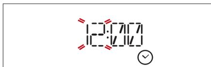
Turn the *adjustment knob* to set the correct hour and press
