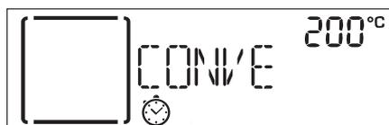
To switch off the timer, turn the *selection knob* to 0 to stop the function that is currently active and then press  $\ll$ .
