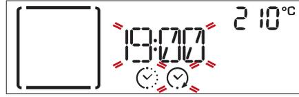
Turn the *adjustment knob* to set the time you want cooking to end, then press  $\frac{OK}{select}$  to confirm and start the function.
