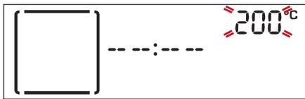
When the value flashes on the display, turn the *adjustment knob* to change it, then press  $\frac{OK}{select}$  to confirm and continue to alter the settings that follow (if possible).
