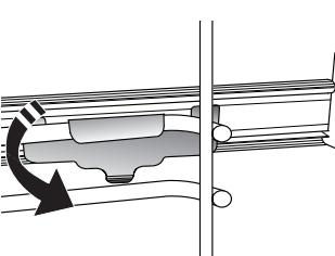
To secure the guide, press the lower portion of the clip firmly against the shelf guide. Make sure that the runners can move freely. Repeat these steps on the other shelf guide on the same level.
