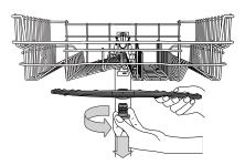
To remove the upper spray arm, turn the plastic locking ring in an anti-clockwise direction. The upper spray arm should be replaced so that the side with the greater number of holes is facing upwards.
