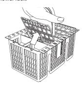
Knives and other utensils with sharp edges must be placed in the cutlery basket with the points facing downwards or they must be positioned horizontally in the tip-up compartments on the upper rack.
