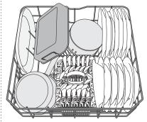
For pots, lids, plates, salad bowls, cutlery etc. Large plates and lids should ideally be placed at the sides to avoid interferences with the spray arm.
