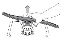
The lower spray arm may be removed by pulling it upwards.
