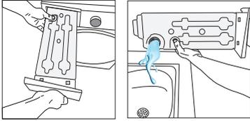
If lint builds up in the funnel on the water tank, remove it under running water. Place back the water tank.
