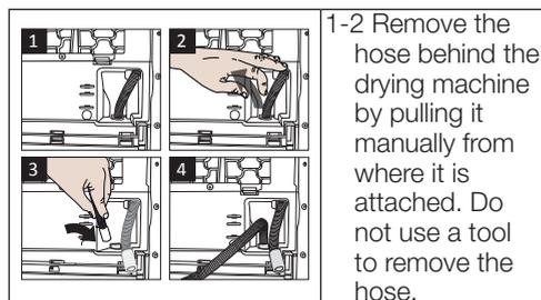
1-2 Remove the hose behind the drying machine by pulling it manually from where it is attached. Do not use a tool to remove the hose.
