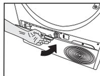
After the cleaning process is completed, place the air deflector cover to its place, move the latches to close it and close the toe board.
