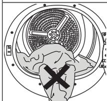
Ensure that no laundry is jammed to the loading door. Do not close the loading door with force.
