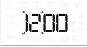
The two digits for the hour will start flashing: Turn the knob to set the hour and then press the central button to confirm.
