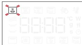
Turn the knob to select from amongst the subfunctions available on the right-hand display and then press the central button to confirm. The sub-function in selection will blink until its confirmation.
