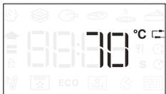
Press **⌚** to start settings. Turn the knob to set the meat probe target temperature. Press **OK** to confirm.
