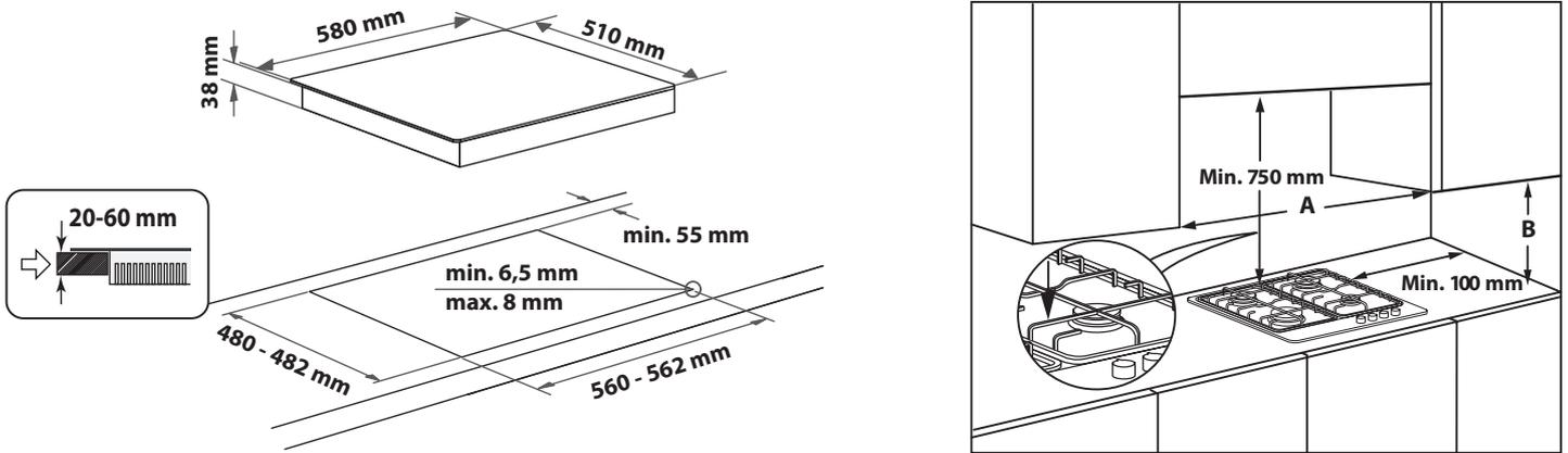
**NOTE:** If distance "A" between the kitchen cabinets is between 600 mm and 730 mm, height "B" must be at least 530 mm. If distance "A" between the kitchen cabinets is greater than the width of the hob, height "B" must be at least 400 mm. If a hood is installed above the hob, refer to the assembly instructions for the hood to see the necessary distance.
