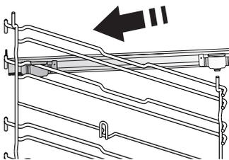
Fasten the upper clip of the runner to the shelf guide and slide it along as far as it will go. Lower the other clip into position.
