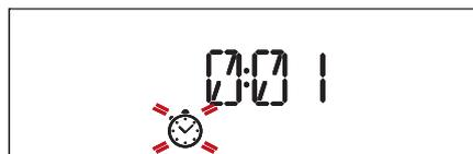
Turn the *adjustment knob* to set the length of time you require and then press the *selection/confirmation button* to activate the timer. An audible signal will sound and the display will indicate once the timer has finished counting down the selected time.
