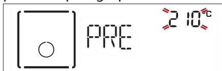
Once this phase has finished, an audible signal will sound and the display will indicate that the oven has reached the set temperature.
