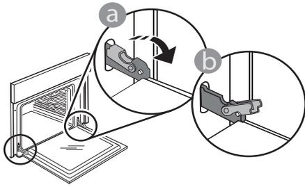
2. Take a firm hold of the door with both hands – do not hold it by the handle. Simply remove the door by continuing to close it while pulling it upwards at the same time until it is released from its seating. Put the door to one side, resting it on a soft surface.
