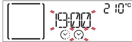
Turn the *adjustment knob* to set the time you want cooking to end, then press the *selection/confirmation button* to confirm and start the function.
