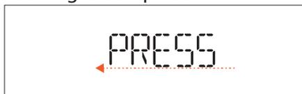
When the display shows the relevant message, if required press the *selection/confirmation button* to start a five-minute browning cycle.
