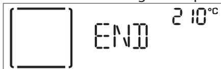
Press the *selection/confirmation button* to continue cooking in manual mode (without a programmed cooking time) or turn the *adjustment knob* to extend the cooking time by setting a new duration.
