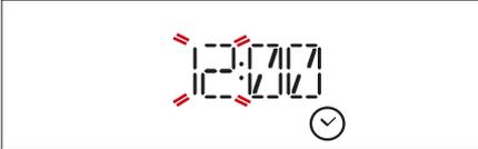
Turn the *adjustment knob* to set the correct hour and press the *selection/confirmation button*: the minutes will flash on the display.
