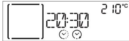
Note: Programming a delayed cooking start time will disable the oven preheating phase: The oven will reach the temperature you require gradually, meaning that cooking times will be slightly longer than those listed in the cooking table.
