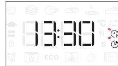
If necessary, turn the knob to set the time you want cooking to end, then press
