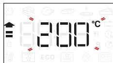
At this point, open the door, place the food in the oven, close the door and start cooking by pressing
