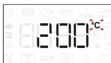
When the °C icon flashes on the display, turn the knob to change the value, then press
