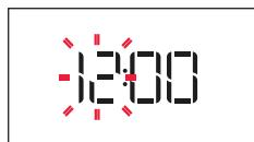
The two digits for the hour will start flashing: Turn the knob to set the hour and press
