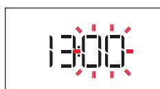
The two digits for the minutes will start flashing. Turn the knob to set the minutes and press
