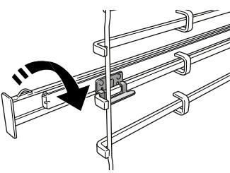
To secure the guide, press the lower portion of the clip firmly against the shelf guide. Make sure that the runners can move freely. Repeat these steps on the other shelf guide on the same level.
