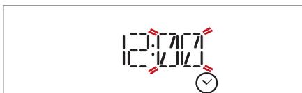
Turn the *adjustment knob* to set the minutes and press **OK select** to confirm.
