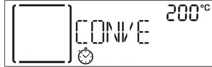
To switch off the timer, turn the *selection knob* to 0 to stop the function that is currently active and then press .
