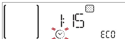
Turn the *adjustment knob* to select the desired cycle and press OK to confirm. The oven begins the self-cleaning cycle, and the door locks automatically: a warning message appears on the display, along with a countdown indicating the status of the cycle in progress.
