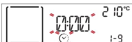
When the **Q** icon flashes on the display, use the *adjustment knob* to set the cooking time you require and then press **OK select** to confirm.
