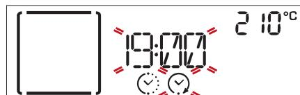
Turn the *adjustment knob* to set the time you want cooking to end, then press **OK select** to confirm and start the function.
