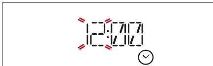
Turn the *adjustment knob* to set the correct hour and press **OK select**: The two digits for the minutes will flash on the display.
