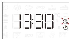
If necessary, turn the knob to set the time you want cooking to end, then press
