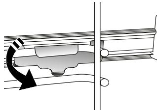
To secure the guide, press the lower portion of the clip firmly against the shelf guide. Make sure that the runners can move freely. Repeat these steps on the other shelf guide on the same level.
