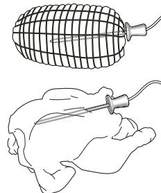
It is very important to position the probe accurately in order to obtain perfect cooking results. Insert the probe fully into the fleshiest part of the meat, avoiding bones and fatty parts. For poultry, the probe should be inserted sideways, in the middle of the breast, taking care to ensure the tip does not end up in a hollow part. In the case of meat with very irregular thickness, check it is cooked
