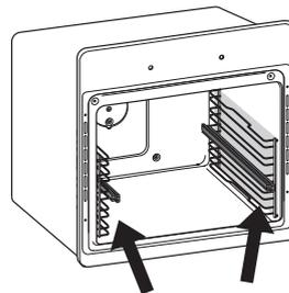
3. Refit the side grilles with the guide rails on the catalytic panels.
