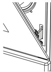
Take a firm hold of the door with both hands – do not hold it by the handle. Simply remove the door by continuing to close it while pulling it upwards at the same time until it is released from its seating.
