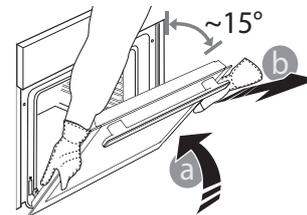
Put the door to one side, resting it on a soft surface. Reversely perform respectively what you did while opening door to reinstall oven door back.
