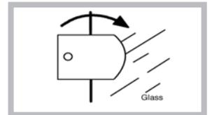
2. Turn the two securing brackets back to their original position to retain the glass and tighten the screws (Fig. 2.)
