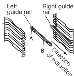
2. Choose which shelf to use with the sliding rack. Paying attention to the direction in which the sliding rack is to be extracted, position joint A and then joint B on the rail.
