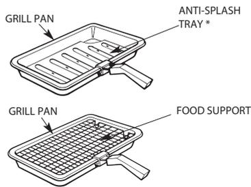
Note: To stop fat splashing onto the grill mesh, it is important to use the anti-splash tray as shown in the grilling chart. Always clean the grill pan, anti-splash tray\* and food support after each use.
