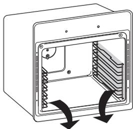
1. To remove the two side grilles, pull them out from the catalytic panels.
