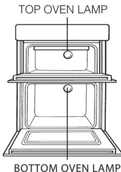
Disconnect the oven from the power supply. Unscrew the cover from the light, replace the bulb (25W - 230V - T 300 °C - E14) and screw the cover back on the light. Reconnect the oven to the power supply.
