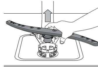
The lower spray arm may be removed by pulling it upwards.
