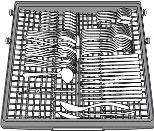
The third rack was designed to house the cutlery. Arrange the cutlery as shown in the figure. A separate arrangement of the cutlery makes collection easier after washing and improves washing and drying performance.
