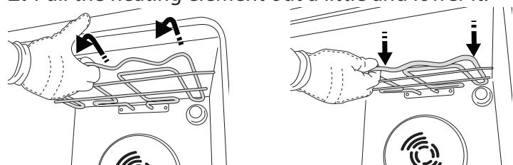
3. To reposition the heating element, lift it up, pulling it slightly towards you, making sure it comes to rest on the lateral supports.
