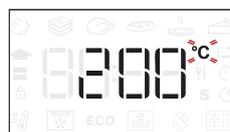
When the °C icon flashes on the display, turn the knob to change the value, then press to confirm and continue to alter the settings that follow (if possible).
