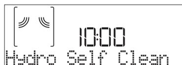
Press  to activate the cleaning function: the display will prompt in sequence actions to be performed before starting the cleaning. Press  anytime when done.
