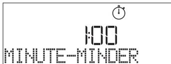
Once the minuteminder has been activated, you can also select and activate a function. Turn the *selection knob* to select the function you require.
