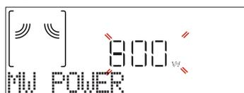
When the value flashes on the display, turn the *adjustment knob* to change it, then press  to confirm and continue with the settings that follow (if possible).
