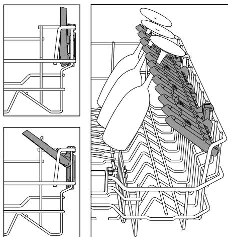
The side foldable flaps can be folded or unfolded to optimize the arrangement of crockery inside the rack. Wine glasses can be placed safely in the foldable flaps by inserting the stem of each glass into the corresponding slots.
