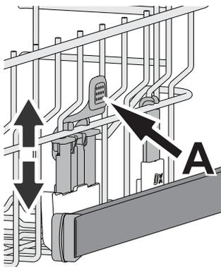
The height of the upper rack can be adjusted: a high position to place bulky crockery in the lower basket and a low position to make the most of the tip-up supports by creating more space upwards and avoiding collision with the items loaded into the lower rack.
