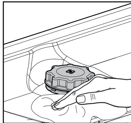
Make sure the cap is screwed on tightly so that no detergent can get into the container during the wash program (this could damage the water softener beyond repair).
