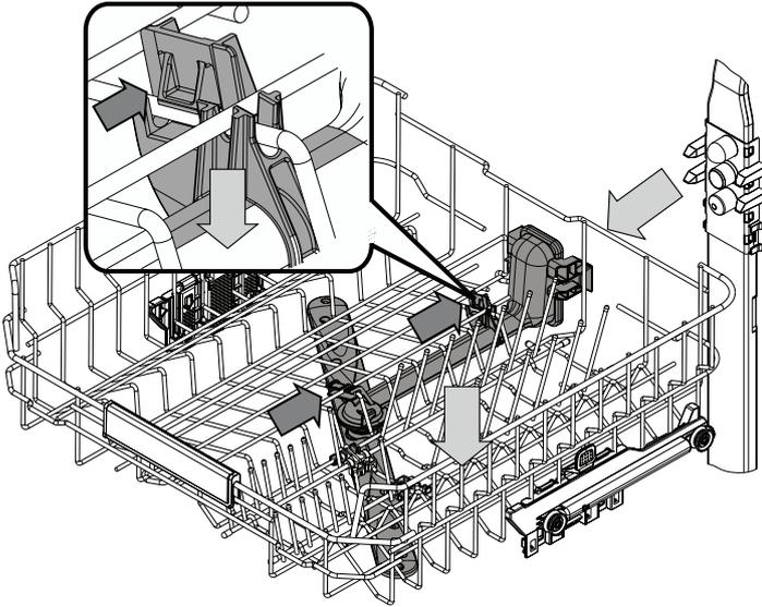
On occasions, food residue may become encrusted onto the spray arms and block the holes used to spray the water. It is therefore recommended that you check the arms from time to time and clean them with a small non-metallic brush.
