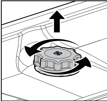
2. Position the funnel (see figure) and fill the salt reservoir right up to its edge (approximately 0,5 kg); it is not unusual for a little water to leak out.
