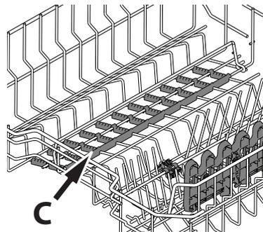
The upper basket contains a special silicone overlay **C** that protects delicate items, such as glassware, from potential damage caused by contact with the rack's prongs.
