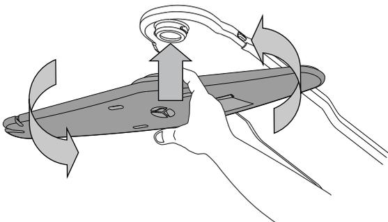
The ceiling sprayer arm may be removed by pressing it up and then rotating it anti-clockwise. Mounting back the spray arm is by pulling it upwards and rotating it clockwise.
