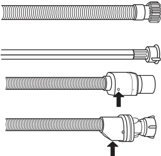
If the inlet hose has a transparent coating, periodically check if the colour intensifies locally. If yes, the hose may have a leak and should be replaced. For water stop hoses: check the small safety valve inspection window (see arrow). If it is red, the water stop function was triggered, and the hose must be replaced by a new one. For unscrewing this hose, press the release button while unscrewing the hose.
