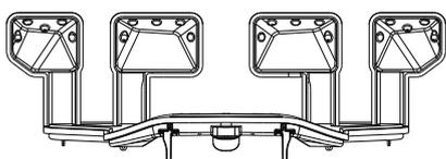
PowerClean Pro uses the special water jets in the rear of cavity to wash more intensively the high dirty items.
