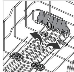
To unfold the tip-up supports, pull them until you hear a click, which means the support has been securely locked in place by the catch. This allows you to easily adjust the space in the rack.
