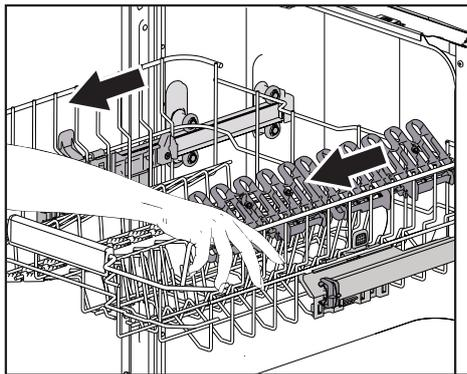
2. Use a soft brush or damp cloth to remove any food residues and dirt accumulated on the rails.
