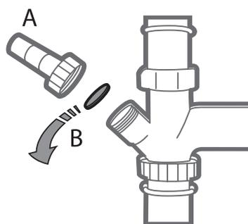
Connect the outlet hose to a drain duct with a minimum diameter of 2 cm **A**.
