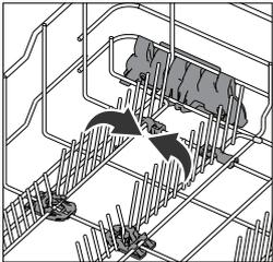
Folding the tip-up supports in the dishwasher rack is simple and quick. To fold the tip-up supports, simply push them in the direction indicated by the arrows on the picture until the catch releases.
