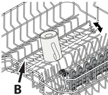
The upper basket is equipped with an additional wire **B** that, when raised to a vertical position, makes it easier to arrange dishes.
