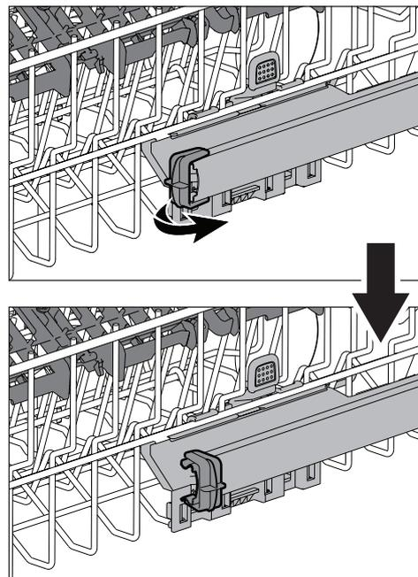
Pull the rack towards you. Completely remove the rack from the rails to the outside.
