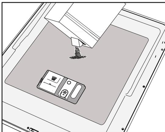
4. Remove detergent residues from the edges of the dispenser and close the cover until it clicks. Close the lid of the detergent dispenser by pulling it up until the closing device is secured in place.
