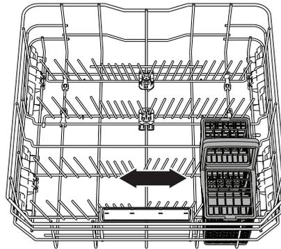
The lower rack has the tip-up supports which can be used in a vertical position when arranging plates or in a horizontal position (lower) to load pans and salad bowls easily.
