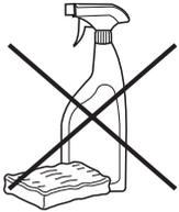
Any marks on the inside of the appliance may be removed using a cloth dampened with water and a little vinegar. The external surfaces of the machine and the control panel can be cleaned using a non-abrasive cloth which has been dampened with water. Do not use solvents or abrasive products.
