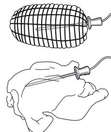
Insert the food probe deep into the meat, avoiding bones or fatty areas. For poultry, insert the probe lengthways into the centre of the breast, avoiding hollow areas.
