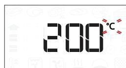
When the  $^{\circ}\text{C}/^{\circ}\text{F}$  icon flashes on the display, turn the knob to change the value, then press to confirm and continue to alter the settings that follow (if possible).
