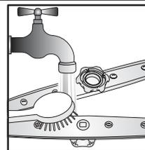
Clean spray nozzles under running water (use toothpicks if necessary)...
