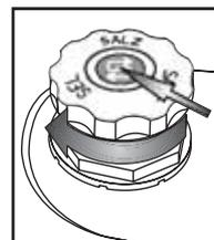
Screw on the cap. Salt residual around the cap need to be removed. Some salt reservoir have a level indicator integrated in the cap (see below how to check).
