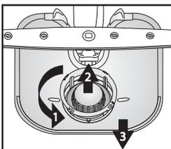
Unscrew microfilter (1), remove it (2) and remove fine sieve (3)...
