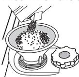
1. Remove the lower rack and unscrew the reservoir cap (anticlockwise).
