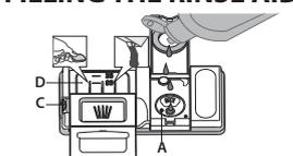
Rinse aid makes dish DRYING easier. The rinse aid dispenser **A** should be filled when the **RINSE AID REFILL** indicator light in the control panel is lit. **NEVER pour the rinse aid directly into the appliance tub.**
