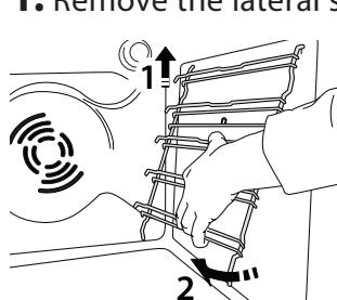
**2.** Pull the heating element out a little and lower it.
