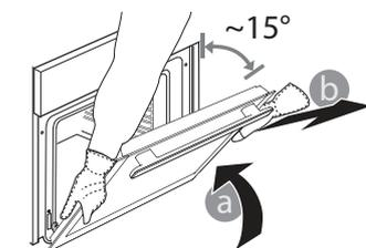
2. Close the door as much as you can. Take a firm hold of the door with both hands – do not hold it by the handle. Simply remove the door by continuing to close it while pulling it upwards at the same time until it is
