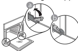
4. Lower the door and then open it fully. Lower the catches into their original position: Make sure that you lower them down completely.
