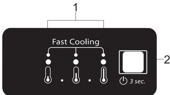
1. Indicator Leds (to display the current temperature setpoint or the Fast Cooling function)
