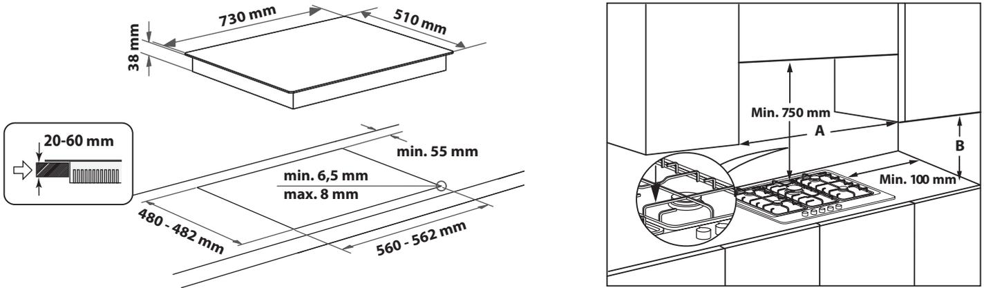
**NOTE:** if distance "A" between the kitchen cabinets is between 600 mm and 730 mm, height "B" must be at least 530 mm. If distance "A" between the kitchen cabinets is greater than the hob's width, height "B" must be at least 400 mm. If a hood is installed above the hob, refer to the hood's assembly instructions to see the necessary distance.
