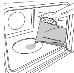
When the oven is cold, fill the recess with the quantity of drinking water suggested in the relevant cooking table. Set and activate the steam·
