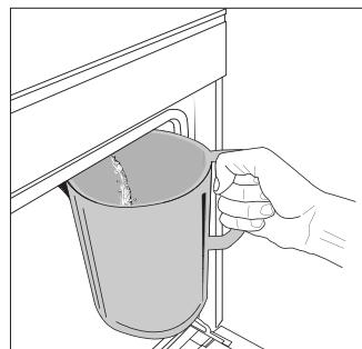
Once selected the "Drain" function or when requested from display, start the function and follow the actions indicated: Open the door and place a large jug (at least 2 liters capable) under the drain nozzle located at the bottom of the panel, to the left of the inlet nozzle. If needed, it is possible operate the control panel to pause the drain process and to resume it (for example in case the jug would be already full of water in the middle of the draining process).
