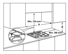
NOTE: if distance "A" between the kitchen cabinets is between 600 mm and 730 mm, height "B" must be at least 530 mm. If distance "A" between the kitchen cabinets is greater than the hob's width, height "B" must be at least 400 mm. If a hood is installed above the hob, refer to the hood's assembly instructions to see the necessary distance.
