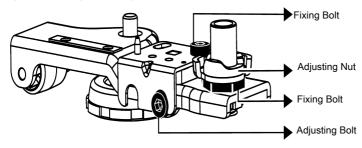
Fix the upper hinge assembly with 3 screws.
