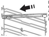
Fasten the upper clip of the runner to the shelf guide and slide it along as far as it will go. Lower the other clip into position.
