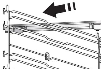
Remove the shelf guides from the oven and remove the protective plastic from the sliding runners.
