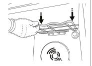
**3.** To reposition the heating element, lift it up, pulling it slightly towards you, making sure it comes to rest on the lateral supports.
