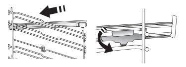
Please note: The sliding runners can be fitted on any level.
