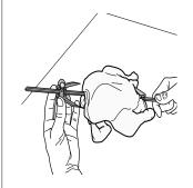
Push the skewer through the centre of the meat (bound with string if poultry) and slide the meat onto the skewer until it is positioned firmly on the fork and cannot move. Push the second fork onto the skewer and slide it on until it holds the meat firmly in place. Tighten the fixing screw to secure it in position.
