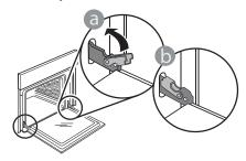
Apply gentle pressure to check that the catches are in the correct position.
