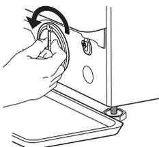
4. Remove filter: Lay a cotton cloth beneath the water filter, which can absorb a small amount of rest water. Then remove the water filter by turning it out anticlockwise.
